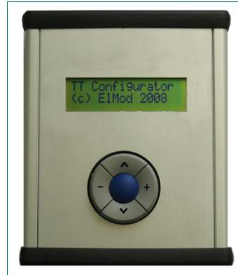
The Configurator shows the name of the connected control unit and its firmware version. Press a key on the key field to get to the first entry of the menu structure. The function of the keys is as follows:
